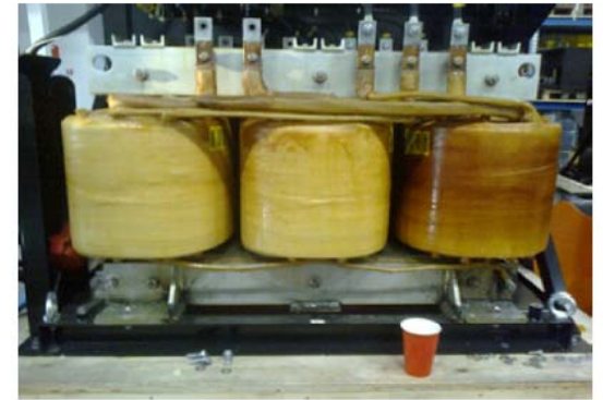
50Hz transformer - 102kVA - 410kg
